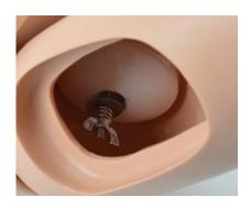
Assemble in this order: washer, spring, and wing nut.
