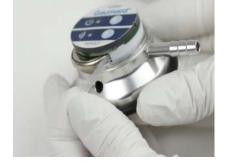
3. Locate the small stereo jack on the bell and attach the speakers provided. Plug the speakers into a conventional 120V/60 Hz wall outlet and turn the speakers on.
